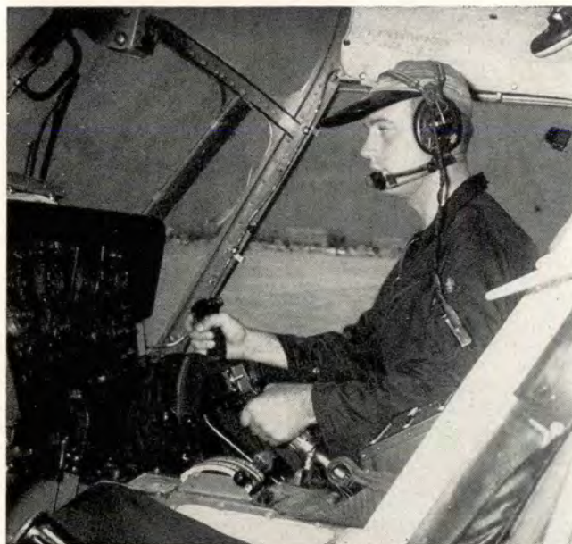
Both hands must be used constantly in the helicopter. The left hand is on the collective pitch stick and throttle.
