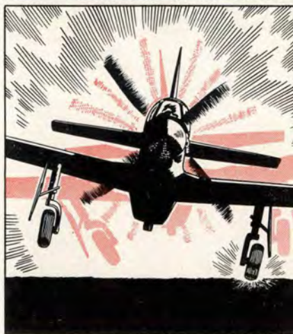
....WAITING UNTIL HE "HAD IT MADE" HE LOWERED THE GEAR....THE RIGHT GEAR FAILED TO LOCK....HE BOUNCED THE LEFT GEAR ALONG THE RUNWAY THUS LOCKING THE RIGHT GEAR IN PLACE!
