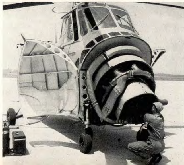
Clam shell doors make the H-19 engine readily accessible.
